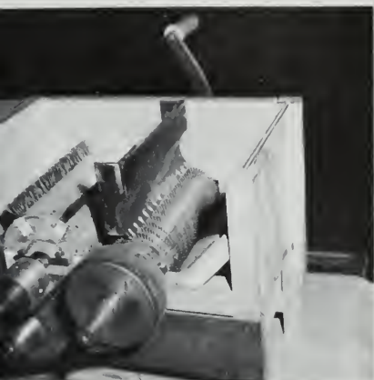
A model of Eli Whitney's gin, built in the shops of the Cotton Ginning Research Laboratory, Stoneville, Miss.
